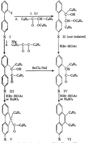
The chlorine-free ketone (IV, X = H) prepared in like manner starting from 2-iodobiphenyl (I, X = H) was found to cyclize more readily than its chlorine-containing counterpart (IV, X = Cl), an effect which might be predicted from the known deactivating influence of a halogen substituent on an aromatic nucleus,<sup>9</sup> as well as the previously observed difficulty in effecting cyclization *meta* to a chlorine atom.<sup>10</sup>
